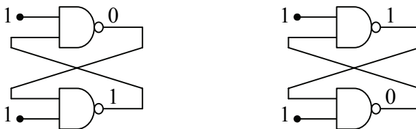
Figure 10-6 Only Two Possible States of Circuit in Figure 10-5
