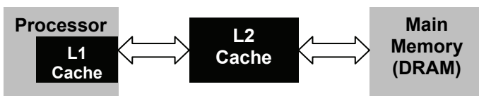
Figure 13-14 L1 and L2 Cache Placement
